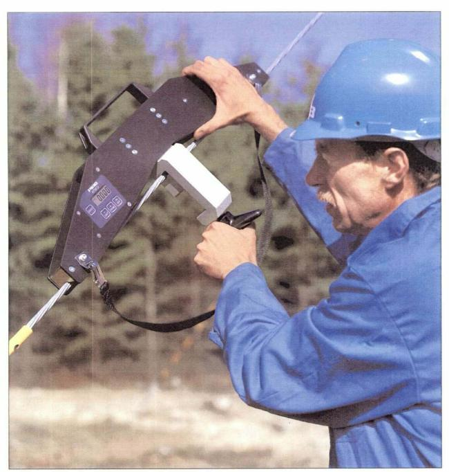
The RTM 20D can be used in applications where accurate measurement in pre loaded wire ropes is required. Such applications can be stay ropes, suspension ropes, catenary ropes etc. The RTM 20D is applied direct to the rope and the measured tension value is presented digitally.
