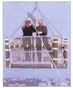
The PIAB RTM 20D is in use when installing/inspecting suspention and catenary ropes.
